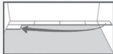
**Fig 6.** General distances between short ends Minimum distance between short ends of planks in parallel rows shall not be less than 500mm. This is for stability of the floor.
