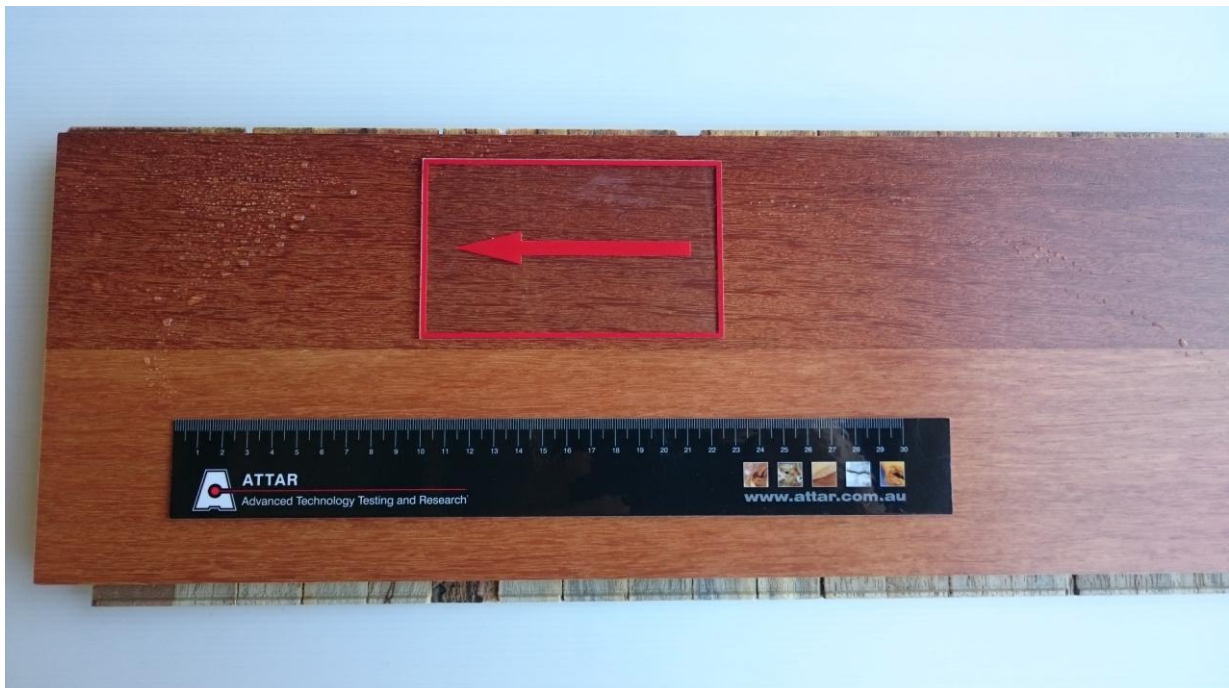
Figure 1: Unilin Engineered wood floor Low Sheen. Highlighted area indicates direction of test.
