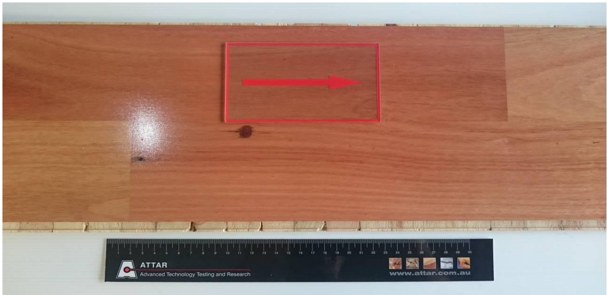
Figure 1: Unilin Engineered wood floor semi-gloss. Highlighted area indicates direction of test.
